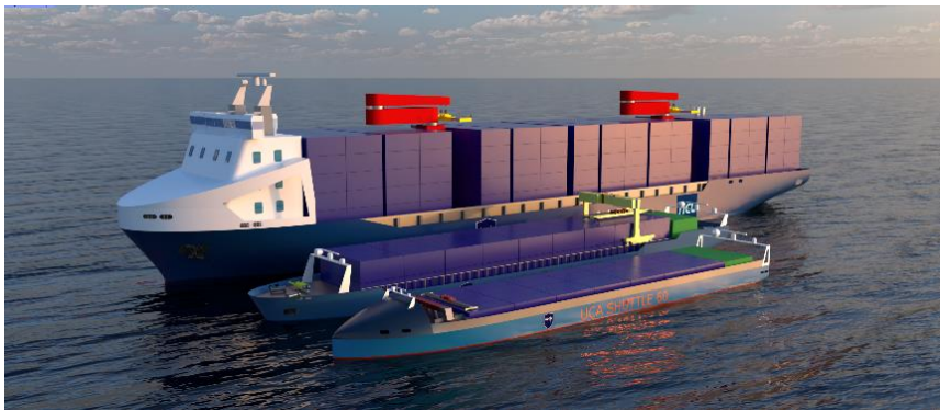
Figure 2: Mother–daughter vessel concept of use case A. 1100 TEU mother vessel, 100 TEU and 60 TEU- shuttles
