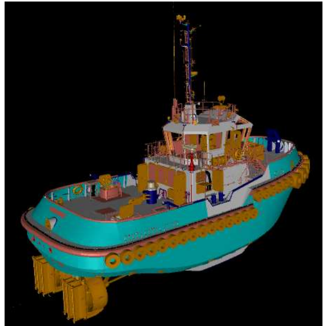
Figure 2. The 3D CAD model of EGE 2, 20.4 m tugboat.
