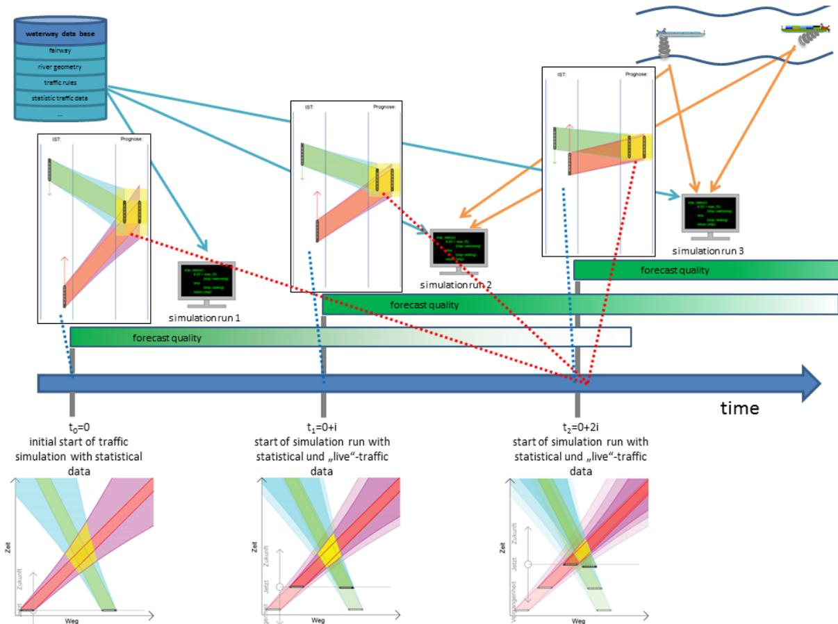
Figure 2: Cascaded runs of traffic simulation to obtain highest forecast quality
